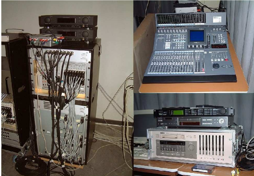
Figure 2.5 DSP, mixer and amplifiers, for the 160 speaker WFS system at the TU Delft
